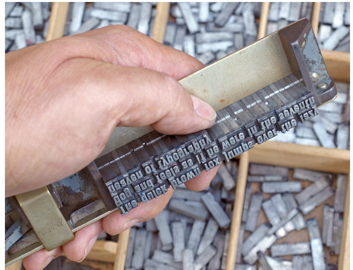
The small pieces of metal type, visible in the background in their typecase, are placed in a small metal tray called a composing stick. Lines of text are composed on the stick and then transferred to a metal frame called a printing form. The form is locked into the press, and pages are printed from it.
