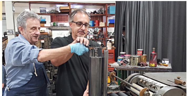
Carl Nudi (left) assists a student at the Tampa Book Arts Studio as they clean the plate cylinder from an offset press.
