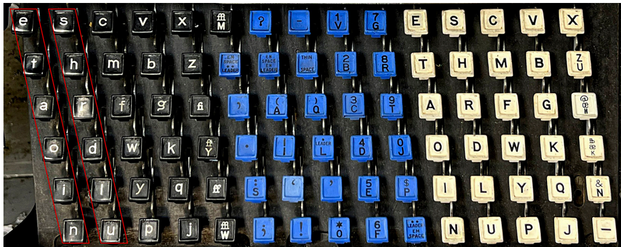
Layout of the Linotype keyboard. Black keys are lowercase letters and ligatures. Blue keys are numerals, some small capital letters, and punctuation. White keys are more uppercase letters and special characters. Note the two columns of keys on the left that spell “etaoin shrdlu,” which became the nickname for the keyboard and the culture of its operators.
